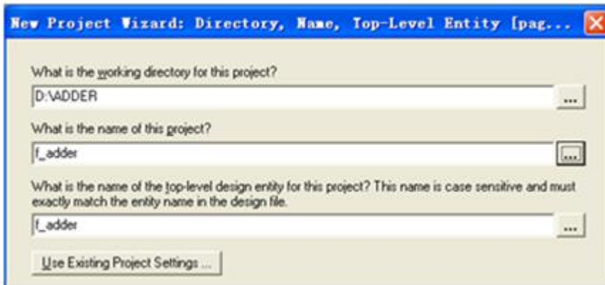
Figure: Full adder f_adder.bdf project settings
